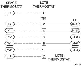
Fig. 47 - Space Thermostat Connections
